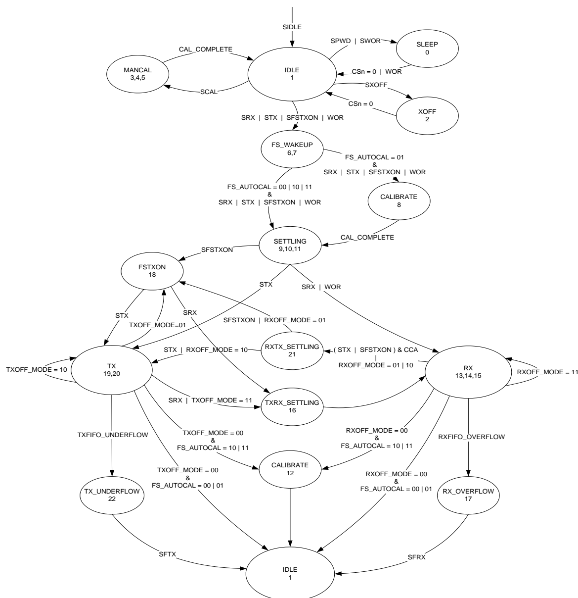
Figure 25: Complete Radio Control State Diagram
