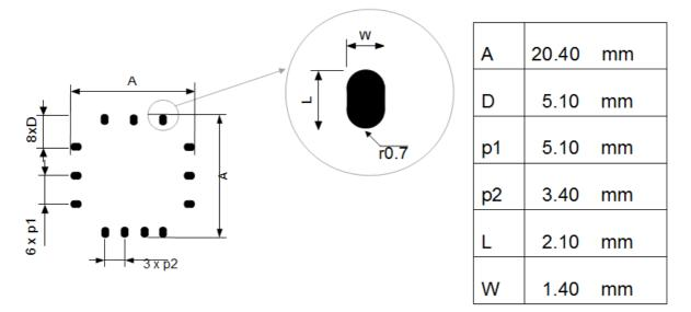
The area underneath the module should be covered with solder resist in order to prevent short circuiting the vias on the back side of the module. A solid ground plane is preferred.
