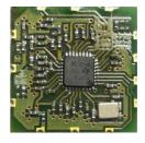
**BITxxxRTH** provides extensive hardware support for packet handling, data buffering, burst transmissions, clear channel assessment, link quality indication and wake-on-radio.
