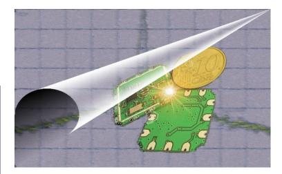
Very low cost transceiver module designed for very low power wireless applications in a very small package (20x20 mm)
