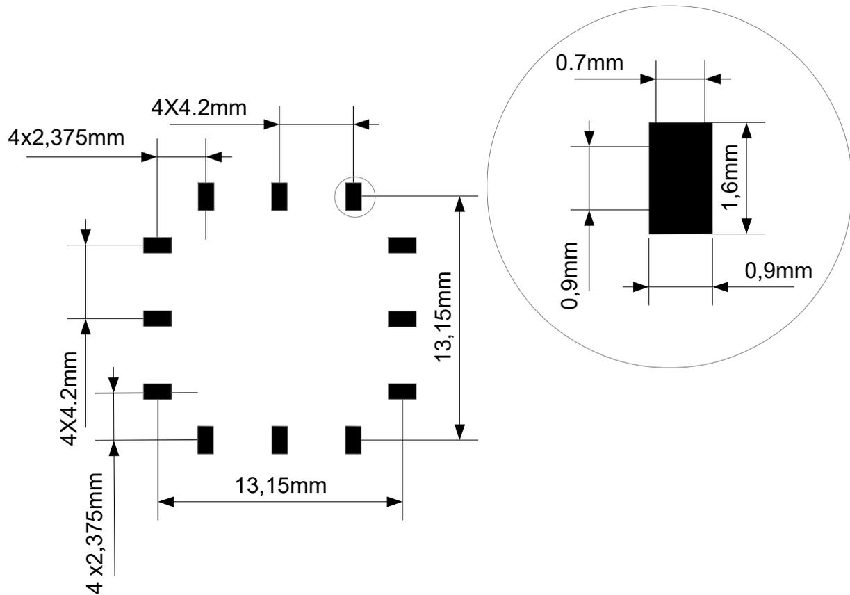
A PCB with two or more layers and with a solid ground plane in one of the inner-or bottom layer(s) is recommended. All GND-pins of the module shall be connected to this ground plane with vias with shortest possible routing, one via per GND-pin
